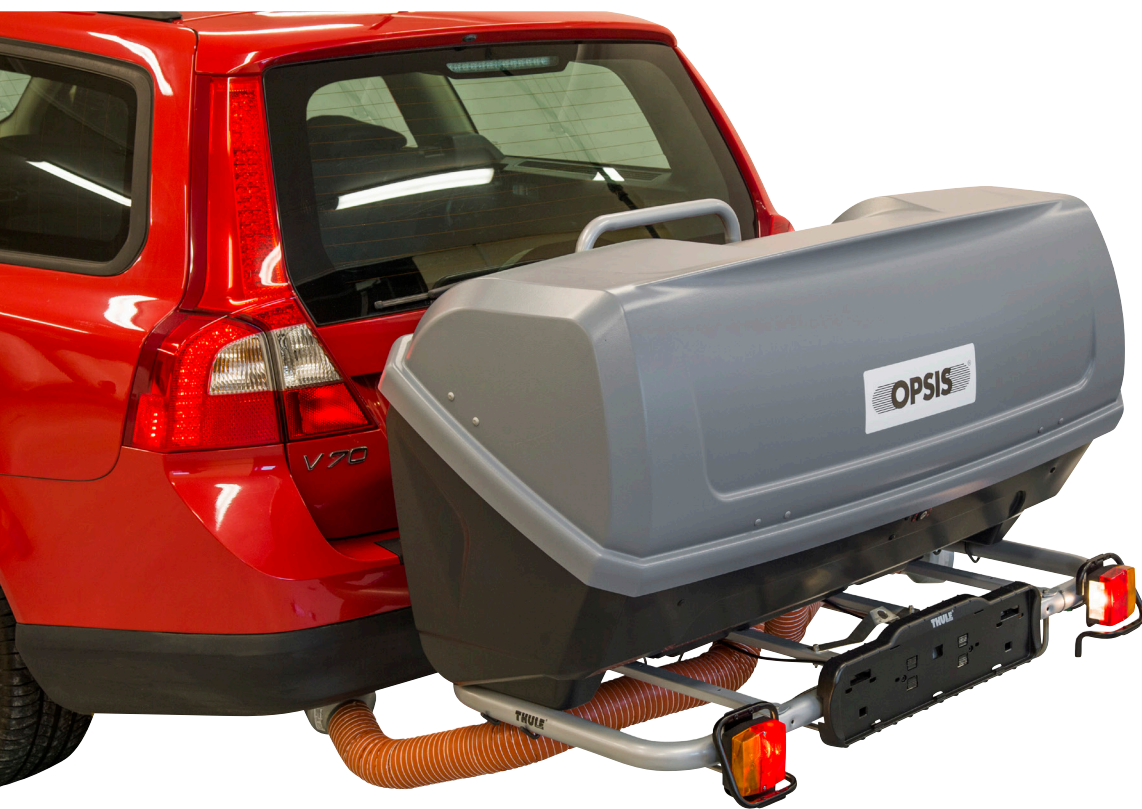
An OPSIS RDE installation.
